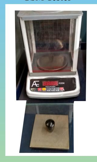
This equipment measures and directly indicates substance of paper and fabric in terms of grams per sq. meter (GSM). It displays gsm of samples cut selected to size on a digital indicator. This GSM value can be used in Bursting Strength Tester to get the burst factor of any paper or boards which is an important factor in the packaging industry, this instrument is used to measure paper GSM, Fabric GSM Tests.
