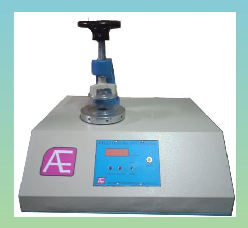
"AKASH" Burst tester is used for accurate measurement of Bursting strength of paper, paper boards, fiber board, filters cloth / Industrial fabric etc. and is manufactured as per national and various international standards. Available with single or double head for testing materials of lower and higher range accurately. Change over from one head to the other by use of two needle valves fitted with the head.
