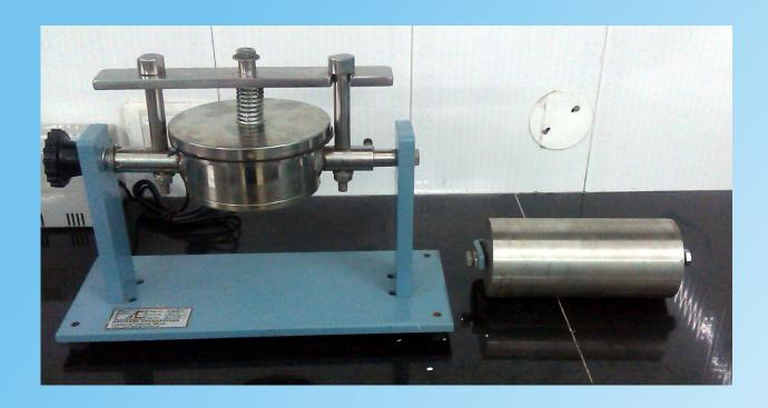
It consists of a cylinder of known inside diameter and length. It has a metallic plate, which is used for clamping the one side of the cylinder with the help of bracket and bolts.
