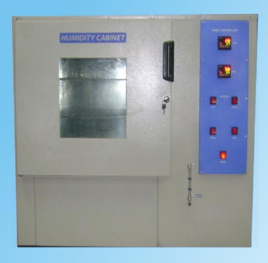
Automated Humidity chamber to determine the effect of relative humidity on sample at various temperatures. The unit is a double walled chamber, with glass wool / PUF insulation. Interior is made of Stainless Steel and Exterior is either made of Mild Steel. The unit has full-length inner glass door and outside metal door with magnetic gasket and lock. The unit is provided with perforated Stainless Steel trays. Forced air circulation for uniform temperature. PU wheels for easy move ability.
