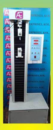
The **AKASH** Digital Universal Tensile Tester is very low cost affordable, low maintenance reliable easy to operate & wide range of applications including: Tensile Testing and Peeling, Flexural, Compression, Shear using appropriate test attachments. On various materials such as Metal Rubber, Plastic, Leather, Asbestos, PVC, Paper, Textile, Wire/Cable, Plywood/wood, Ceramics material etc. in conformity with standards like BIS, ASTM, DIN or ISO.
