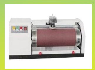
Abrasion tester allows you to measure the abrasion resistance of rubbers (vulcanized thermo-set rubbers and thermoplastic elastomers) that are subject to abrasive/frictional wear in their actual service, such as tyre, conveyor drive belts, and shoe soles.
