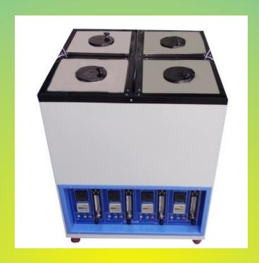
"AKASH" make Multi-cell Ageing Oven suitable for Ageing test of PVC & Rubber as per BS 903 part A 19 method A for rubber. BS 6746 (1976) method E for PVC. It confirms to IS 3400 (Part IV) 1978 Construction: Solid cast aluminum main body.
